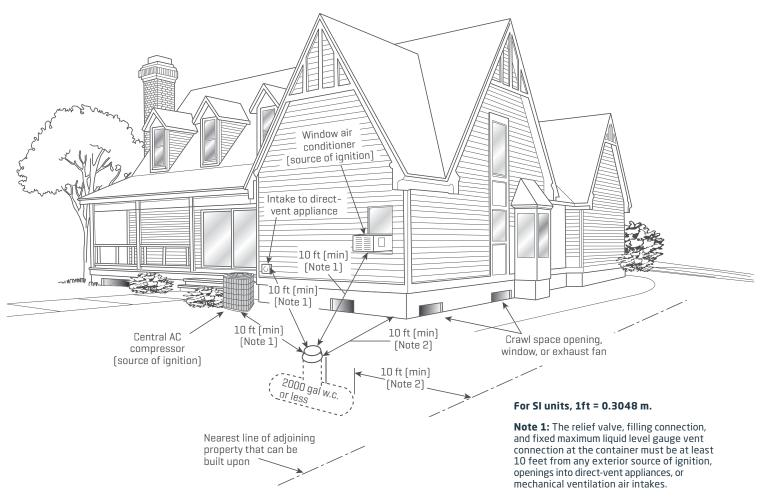
**Note 2:** No part of an underground container can be less than 10 feet from an important building or line of adjoining property that can be built upon.
